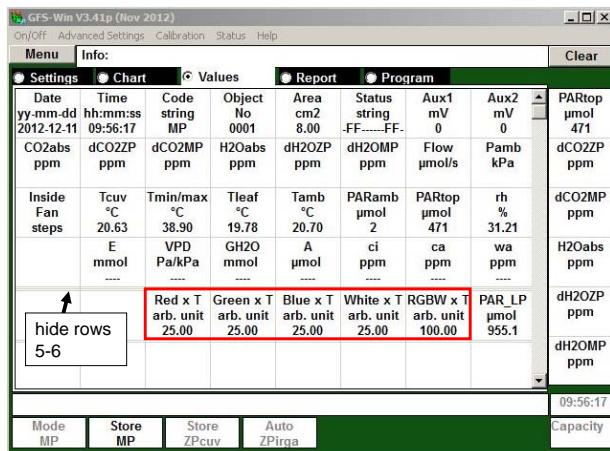
Fig. 6: LED-Panel RGBW values are displayed in row 7 of the values window
