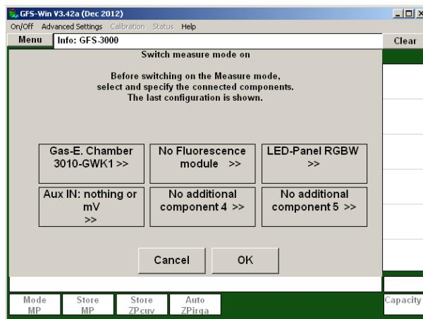
Fig. 2: Choosing Gas-E. Chamber 3010-GWK1 and LED-Panel RGBW in GFS-Win and on the Panel PC
