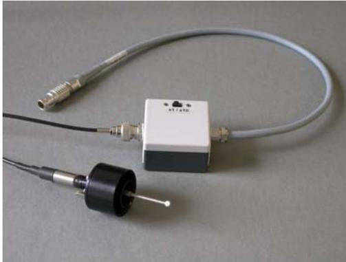
Fig. 5: Spherical Micro Quantum Sensor US-SQS/WB
