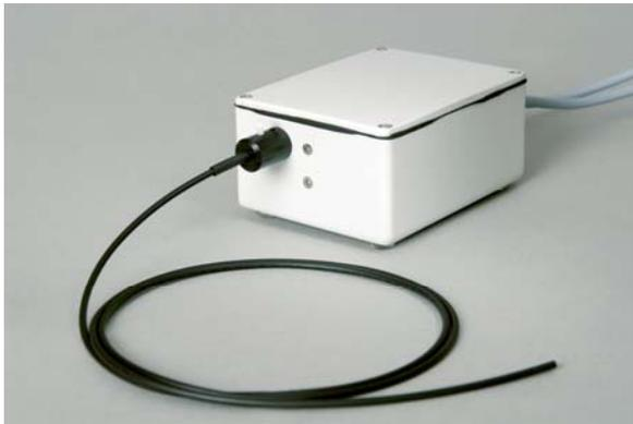
The FIBER version probes surfaces of solid objects by using an optical fiber. Typically the FIBER version is employed to examine photosynthetic layers on various submerged surfaces (periphyton, microphytobenthos) and soil crusts but also to screen samples on
