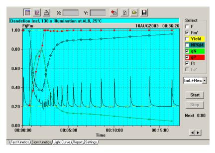
Fig. 10 Example of Induction Curve plus Recovery with display of the fluorescence parameters Fm', qN, qP and Ft
