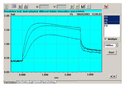
Fig. 11 Fast Kinetics window showing recordings of rapid dark-light induction curves
