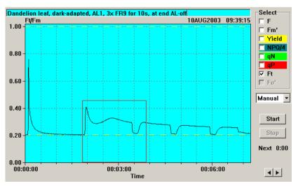
Fig. 8 Example of Manual recording of Slow Kinetics with a part of the recording being marked for Zoom-display
