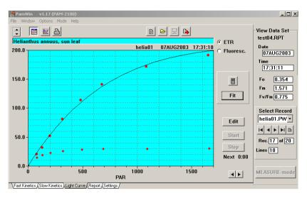
Fig. 13 Light Curve window in the VIEW-mode with display of two superimposed Light Curves
