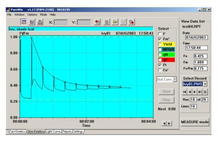
Fig. 14 Slow Kinetics window in the VIEW-mode showing the kinetic information saved in the PWS-file which was recorded in conjunction with one of the Light Curves displayed in Fig. 13
