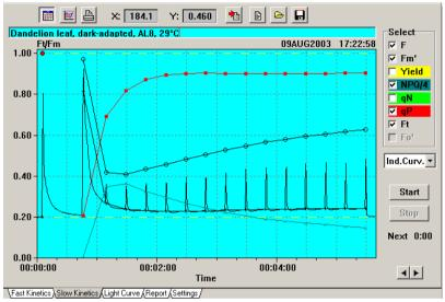
Fig. 7 Slow Kinetics window showing recording of Induction Curve
